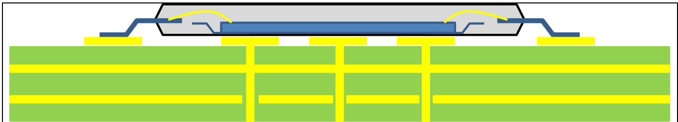
Figure 8-1: Example thermal via holes on PCB.
