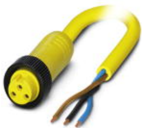
Power cable, 3-position, PVC, yellow, free cable end, A - standard, on Socket straight 7/8"-16UNF, cable length: 2 m
