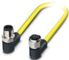
Sensor/Actuator cable, 8-position, PVC, yellow, Plug angled M12 SPEEDCON, A-coded, on Socket angled M12 SPEEDCON, A-coded, Cable length: 1.5 m
