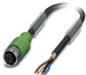
Sensor/actuator cable, 4-position, Variable cable type, shielded, free cable end, on Socket straight M12, A-coded, cable length: Free input (0.2 ... 40.0 m)
