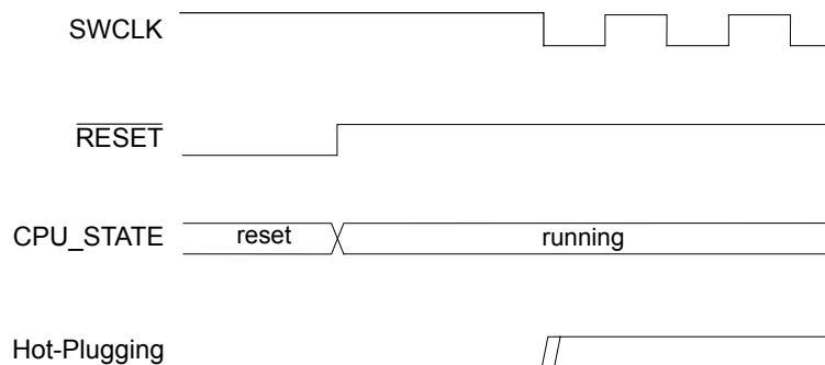
Figure 15-3. Hot-Plugging Detection Timing Diagram
