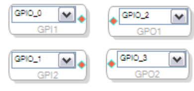
Figure 12. GPIO Input and Output Blocks in SigmaStudio
