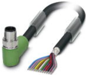
Sensor/Actuator cable, 12-position, PUR/PVC, Black RAL 9005, shielded, Plug angled M12 SPEEDCON, A-coded, on free cable end, Cable length: 1.5 m
