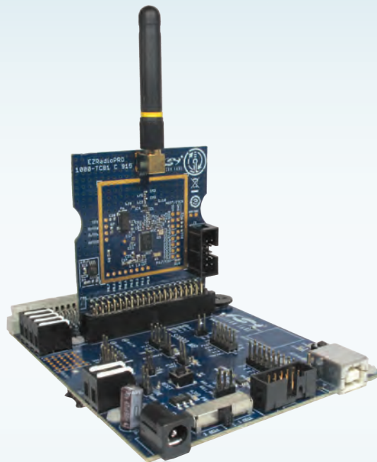
Si1000 TARGET BOARD WITH EZRadio® TEST CARD
