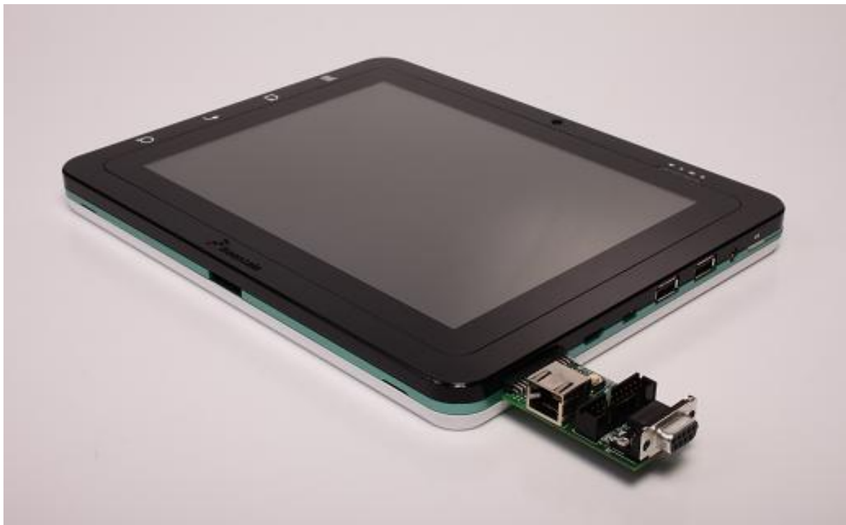
Figure 1-1. MCIMX53SMD Board with a Debug Card and a Display
