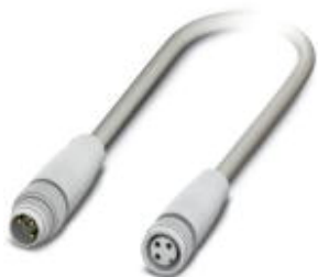
Sensor/Actuator cable, 3-position, PP-EPDM halogen-free, gray RAL 7035, Plug straight M8, on Socket straight M8, Cable length: 0.6 m, Hygienic design, with plastic knurl
