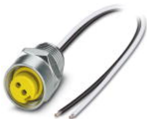
Flush-type connector, 2-position, Socket, straight, 7/8"-16UNF, on free cable end, Front mounting, with 1/2 inch-14 NPT mounting thread, Individual wires, cable length: 1 m
