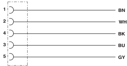
Contact assignment of the M12 sockets
