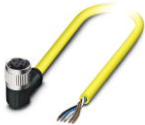
Sensor/actuator cable, 5-position, PVC, yellow, free cable end, on Socket angled M12 SPEEDCON, A-coded, cable length: 5 m
