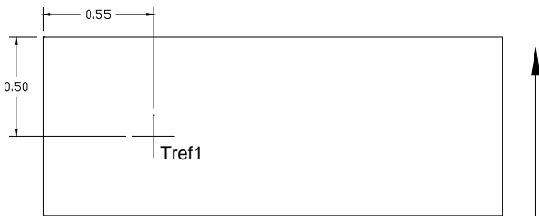
Figure 18. Case ( T_{REF} ) Temperature Measurement Location (top view).
