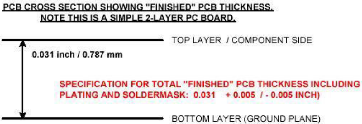
Figure 7. Cross-Section of +12 Volt Striplight PCB.
