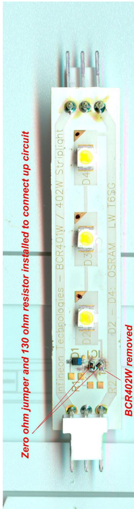
Figure 13. Photo of a 12 Volt Striplight PCB, modified by removing the BCR402W LED Driver IC, and replacing the BCR402W with a 130 ohm resistor. A zero ohm "jumper" was also needed to complete the connections.
