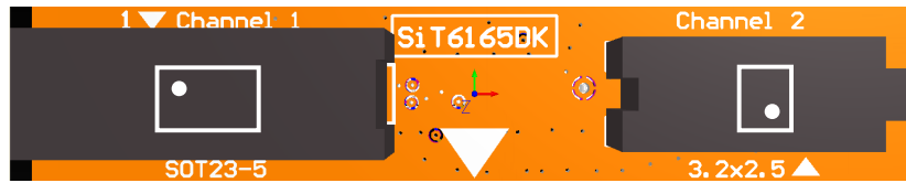
Figure 6: Time Machine socket card SiT6165DK. Supports S package (SOT23-5) and 3.2mm x 2.5mm (6 pin) packages
