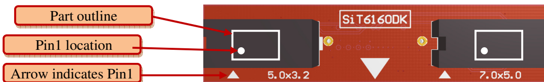
Figure 2: Time Machine socket card SiT6160DK. Supports 5.0mm x 3.2mm (6-pin) and 7.0mm x 5.0mm (6-pin)
