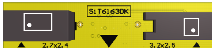
Figure 5: Time Machine socket card SiT6163DK. Supports G package (2.7mm x 2.4mm 4 pin) and 3.2mm x 2.5mm (6 pin) packages
