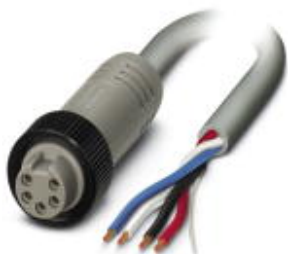
Bus system cable, DeviceNet™, 5-position, PVC, gray, free cable end, A - standard, on Socket straight 7/8"-16UNF, A - standard, cable length: 15 m
