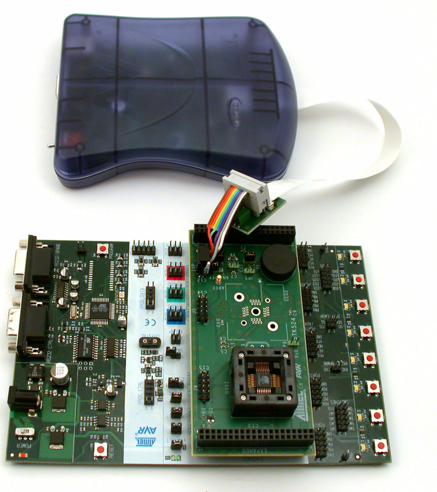
Figure 4-3. Connecting JTAGICE mkII to the STK524
