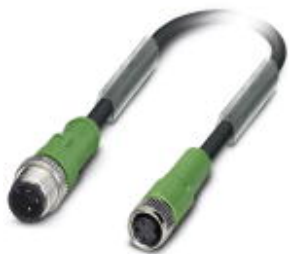
Sensor/actuator cable, 3-position, PUR halogen-free, black-gray RAL 7021, Plug straight M12, A-coded, on Socket straight M8, cable length: 0.3 m
