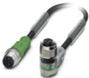
Sensor/actuator cable, 3-position, PUR halogen-free, black-gray RAL 7021, Plug straight M12, A-coded, on Socket angled M12, A-coded, with 2 LEDs, cable length: 5 m
